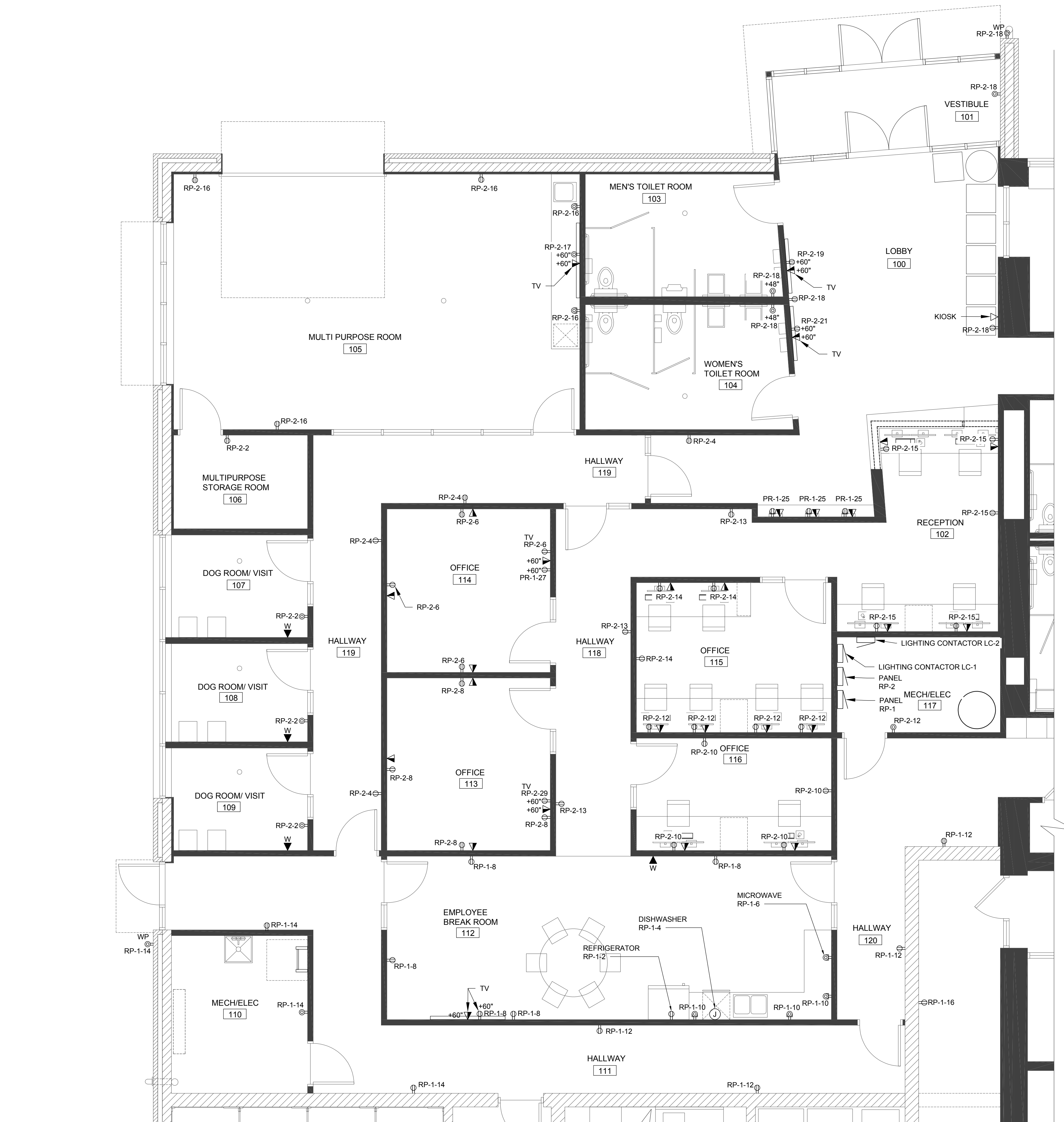
1 ENLARGED ELECTRICAL POWER FLOOR PLAN SCALE: 1/4" = 1'-0"
